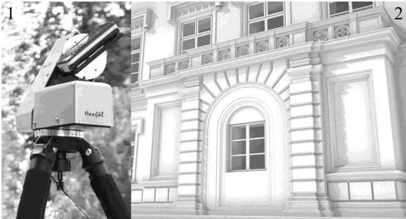
Fig. 1, 2 Flexijet device. 3D model of facade portal of the Royal Palace in Łobzów and the example of architectural inventory, which employs laser measurements in ArchiCAD programme interconnected with Flexijet system.
