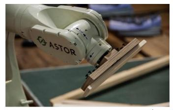
Fig. 1 Creation of the installation with the use of a six-axis robot during the "RÓWNO\_REGLE" (Nationwide Meetings of Architecture Students - OSSA, 2017 Zakopane).
